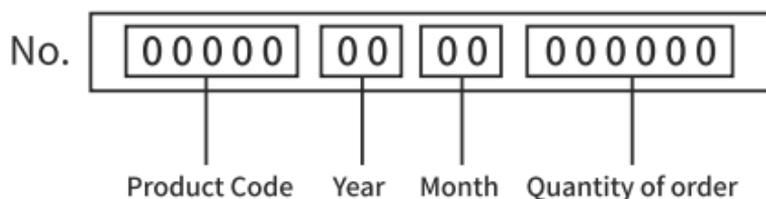
The date of manufacture of the product is encoded in the serial number printed on the body of the tool. The first 2 digits indicate the year of issue, the next 2 digits indicate the month.
